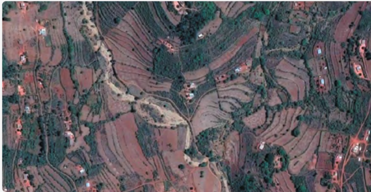
Landscape-scale agroecology, with contoured terracing successfully slowing and sinking surface water run-off, and reducing soil loss and the likelihood of landslides.
